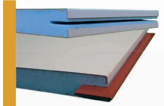
**Panels Specifications** Heat loss coefficients for XPS and PET panels, grooved on 1 or 2 sides U = K = 0.93 (28mm) - 0.82 (32mm) - 0.51 (52mm) W/K.m<sup>2</sup> Heat loss coefficients forLouvered XPS and PET panels on 1 or 2 sides U = K = 0.96 (28mm) - 0.90 (32mm) - 0.54 (52mm XPS uniquement) W/K.m<sup>2</sup>
