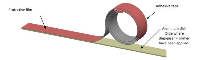
Remove the protective film from the adhesive tape on the aluminum plate that has just been coated:
