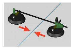
After fitting, push the panel against the top of the upper aluminum profile.
