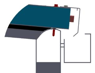
The edge must never touch the key junction. A minimum gap of 10mm must be maintained to allow water to drain properly.
