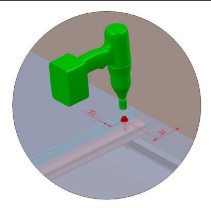
8. Installing the edge profile on the gutter side
