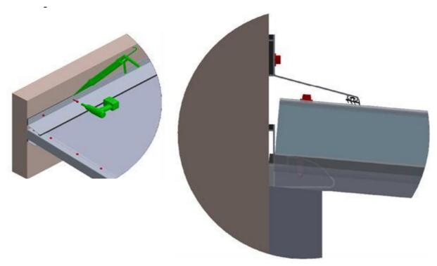
Sheet metal folding is required to ensure watertightness and finish on the sides of the flashing.
