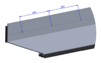
Drill the holes on the bottom wall bracket, spacing each hole 200 mm apart;
